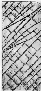
FIG. 175. Arrangement of fractures in glass plate broken by torsion. (Daubrée.)
